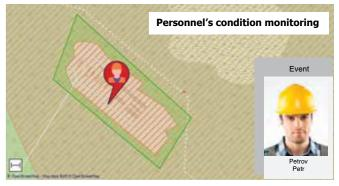
Wearable devices automatically transmit alert to security center in case of worker's loss of consciousness (built-in motion sensor).
