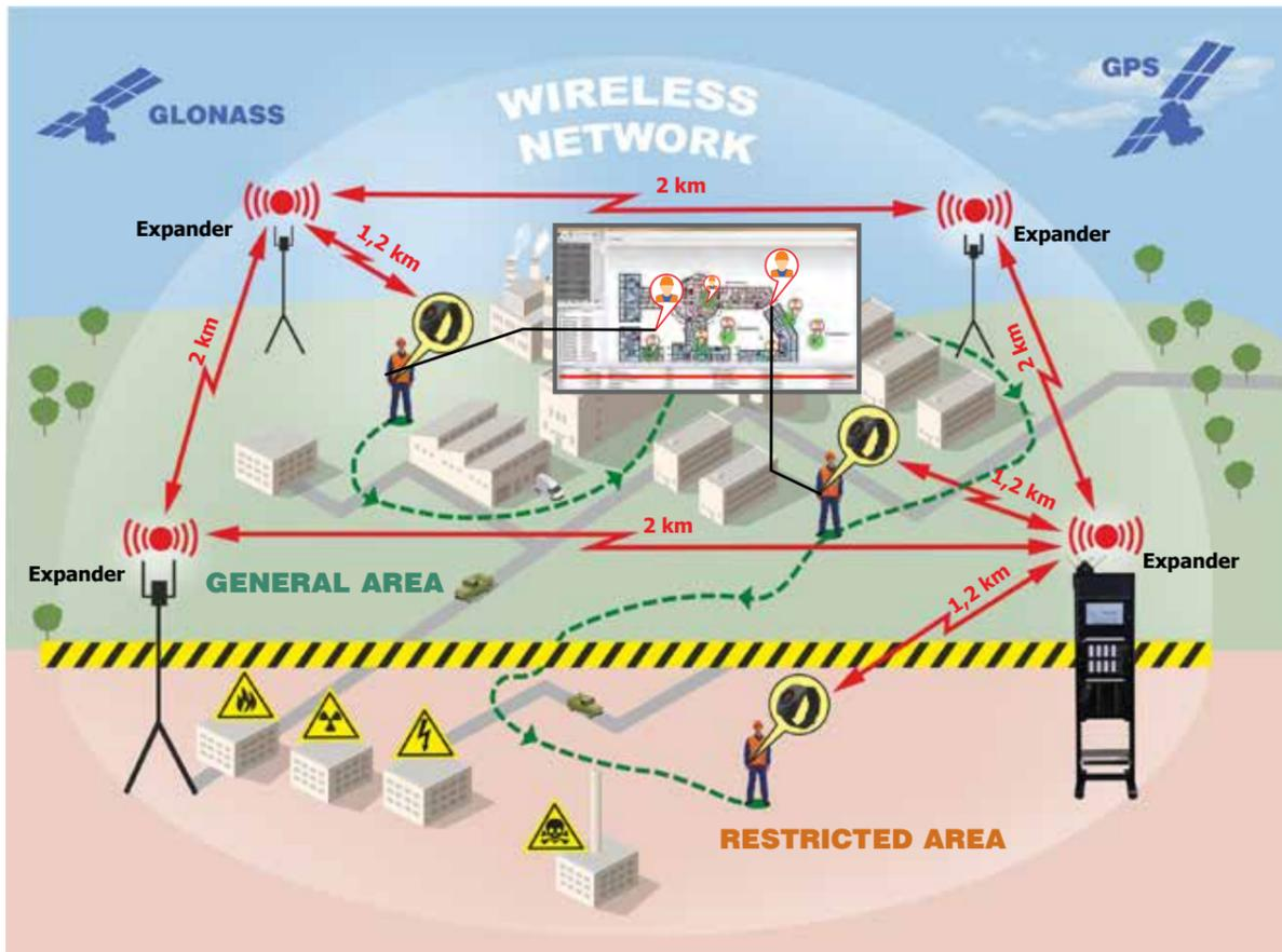
of a portable kit providing alarm and control system for temporary objects
