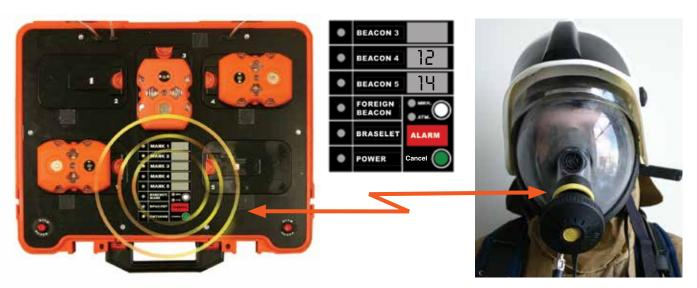
The Mayak Beacon continuously samples the air pressure level in the SCBA cylinder and sends data to the mobile control station. The system evaluates and informs the rescuer team the pressure level in bar units and the remaining amount of air in minutes.
