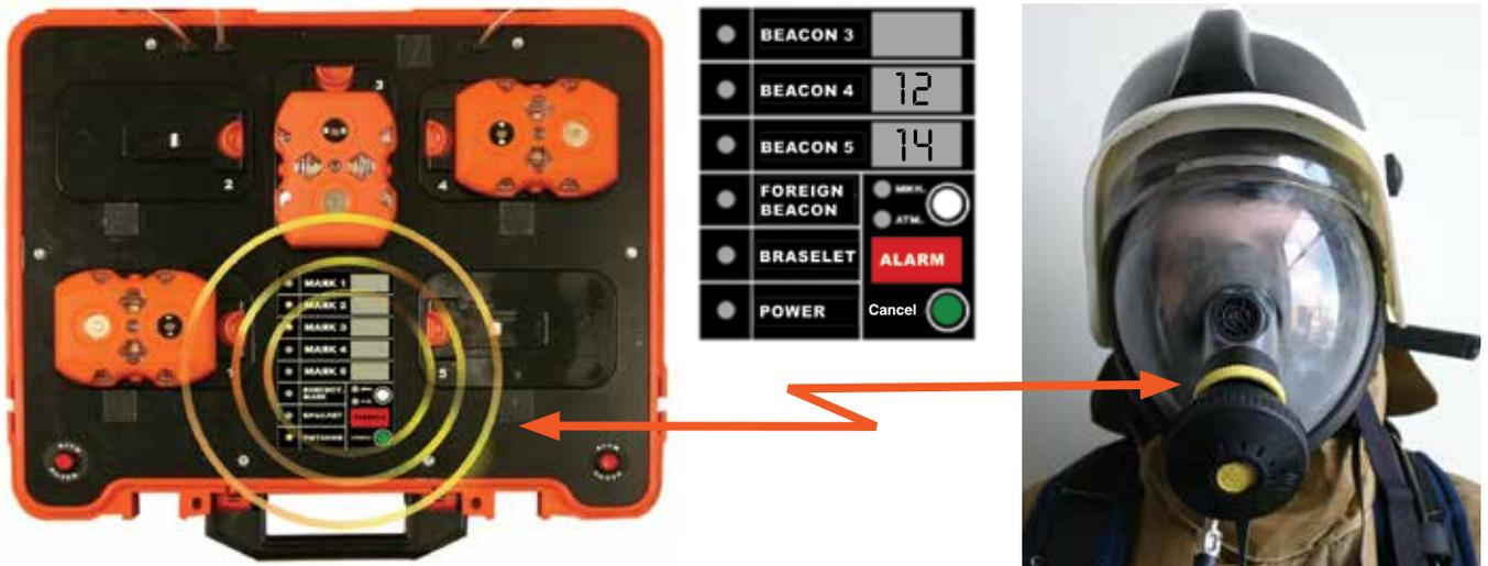
The Mayak Beacon continuously samples the air pressure level in the SCBA cylinder and sends data to the mobile control station. The system evaluates and informs the rescuer team the pressure level in bar units and the remaining amount of air in minutes.
