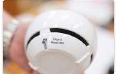
While installing Stretetz-PRO, the existing alarm system can continue to function concurrently. No immediate removal is necessary, given that the wireless equipment doesn't rely on the pre-installed cable lines and circuits. For efficiency, Stretetz-PRO detectors can be set up alongside the old devices, and the old system can be dismantled when it doesn't disrupt the educational process.
